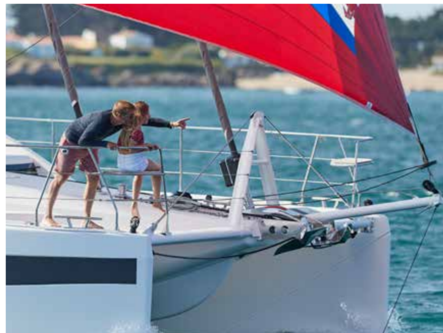
The optional gennaker adds 120sqm of sail to the fully-battened, well-balanced main
