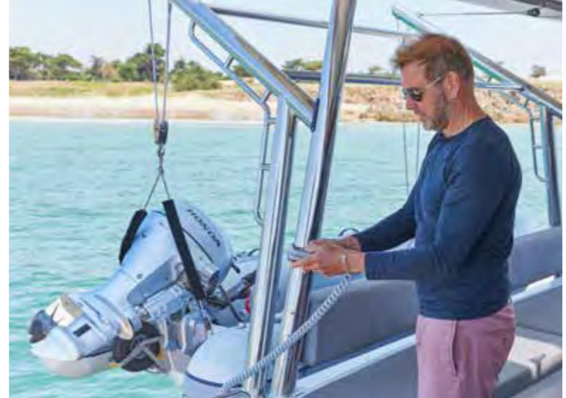
Push-button electric davits make light work of launching and recovering the tender
