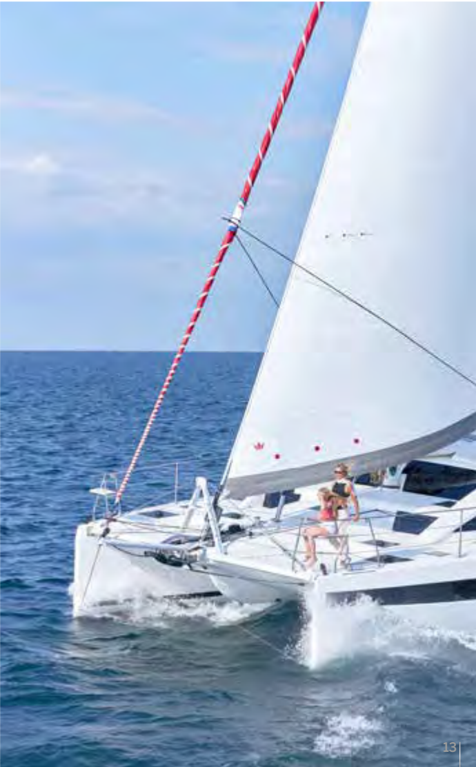
The self-tacking jib is on an electric furler, with a furling gennaker on the elegant bowsprit
