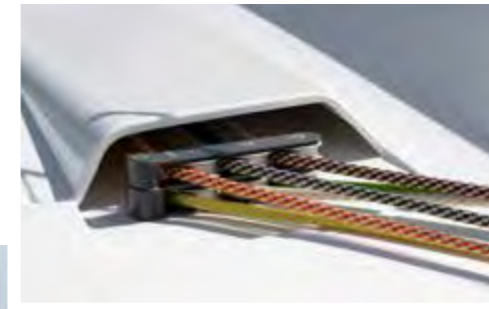
Sheets and halyards are lead to the intuitive helm station. It is easy to sail this boat singlehanded
