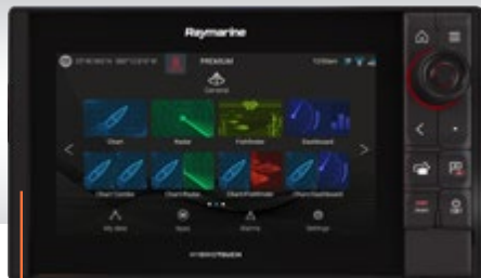
2 Raymarine AXIOM PRO 9 S chart plotter with HybridTouch multifunction display at helm station, stb
